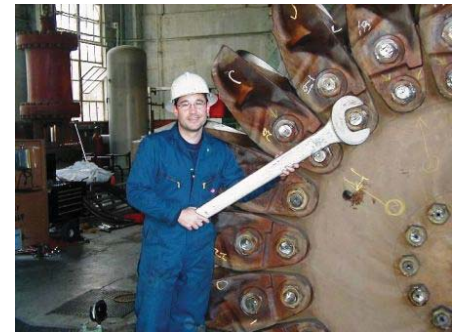
Full size Pelton wheel water turbine at an Hydroelectric powerstation.
